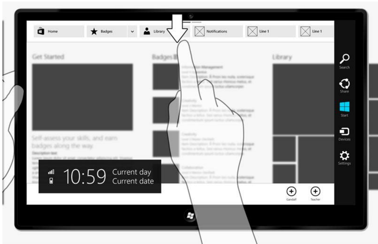
Figure 4. The navigation menu on the Microsoft Surface tablet device. This illustration uses a mockup of the Windows 8.1 operating system. gesture on the bezel of the device, that is a drag down from the bezel into the screen reveals the navigation menu. The low affordance of this menu, the small height of the device’s top bezel, and the limited bezel width that is at reach each moment may hinder its use. Right-clicking when using a mouse reproduces the same behaviour.
